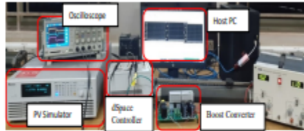
Hardware set up of the PV system.
